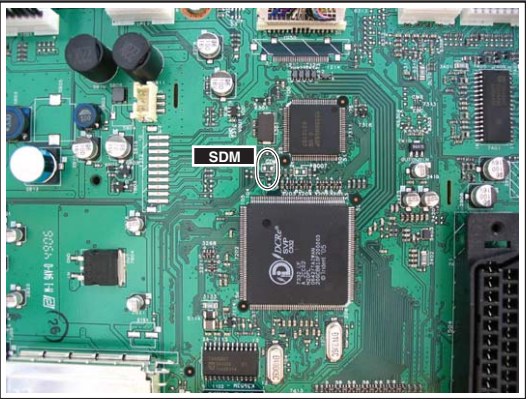
Figure 5-2 Service jumper (SSB component side)
